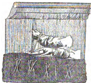
FIG. 2.—Gobelins tapestry-weaving, showing (a) the left hand of the weaver pulling forward (c) a group of warp threads, into which with (b) the comb in his right hand he is compressing at point (d) the weft threads which have been passed around and in between the warp threads; (e) are various bobbins, hanging at rest, suspended by their weft threads; and (f) is the tapestry as woven and compressed.
