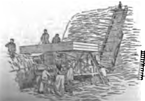
FIG. 2.—Thrashing machine at work with machine elevator behind. (Clayton & Shuttleworth, Lincoln.)
